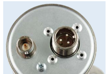
Additional BNC connector for high voltage measurement
