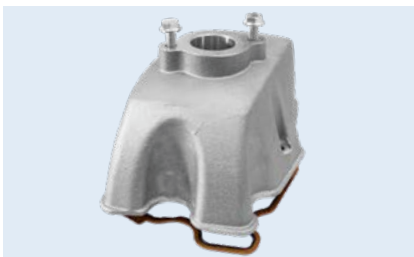
Valve cover with flange support and valve cover gasket
