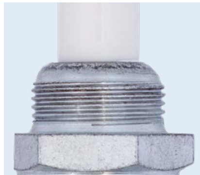
Competitor top threads with only 4 threads do not meet the CSA requirements
