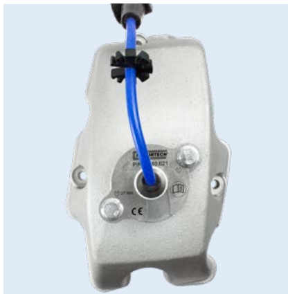
The flanges with the locked spark plug lead are fixed on the valve cover with two screws to prevent the release of components from the spark plug well.
