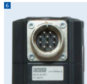
MIL connector for connection to VariStep3 stepper motor driver
