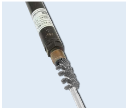
Cleaning of extended barrel spark plug
