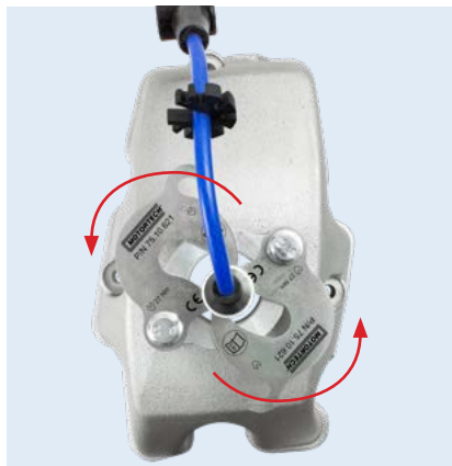
To unlock the spark plug lead the two screws just have to be loosened. The safety flanges can now be turned aside on the flange support.
